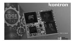
Kontron has expanded its portfolio to include the OSM-S i.MX93 with Dual Core Arm® Cortex®-A55 @1.7 GHz with a 250 MHz Cortex® M33 real-time co-processor, up to 2 GB LPDDR4-RAM and 512 GB eMMC. The module can be directly soldered, allowing it to be assembled, tested and programmed ...
